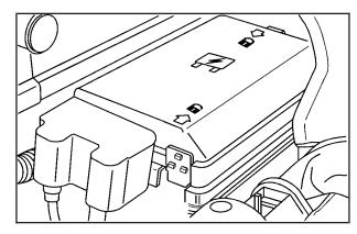
The engine compartment fuse block is located on the driver side of the engine compartment. See *Engine Compartment Overview on page 5-12* for more information on location.
